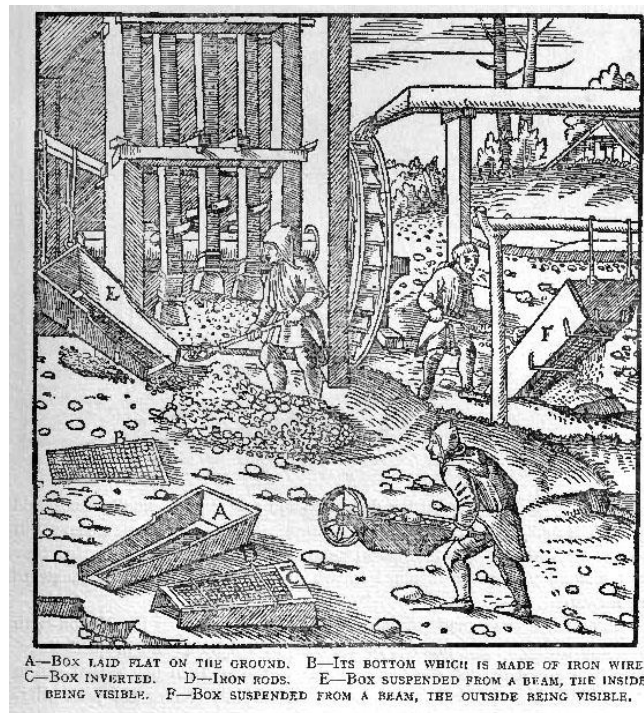
Wood cut from De Re Metallica showing a stamp mill
